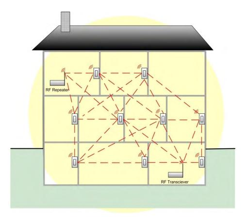
Crestron infiNET Wireless System
